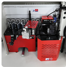
Pre-Milling & Gluing , Pressing Unit
