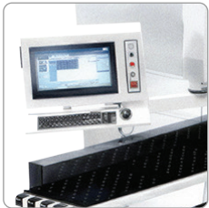
HMI Operator Station
