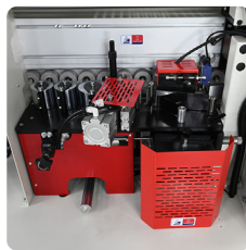
Pre-Milling & Gluing, Pressing Unit
