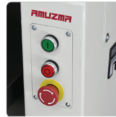
Main Control Panel with Emergency Stop
