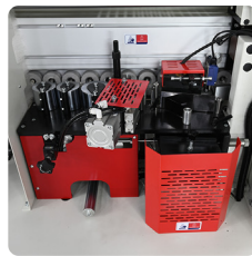
Pre-Milling & Gluing , Pressing Unit
