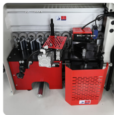
Pre-Milling & Gluing, Pressing Unit
